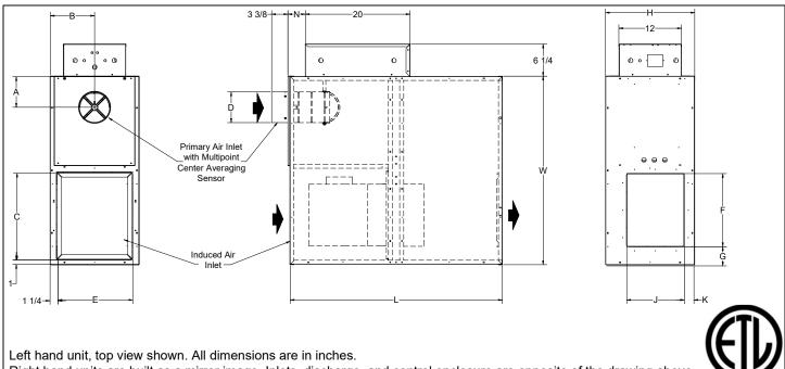
Right hand units are built as a mirror image. Inlets, discharge, and control enclosure are opposite of the drawing above.
